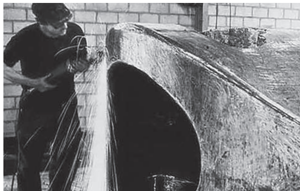
Figure 10. Finishing of a gerberette
