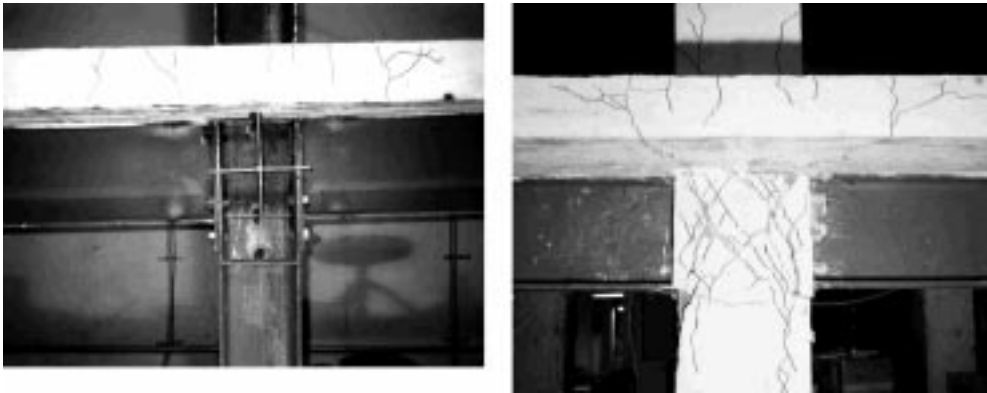
Fig. 11 Photos of the prototypes after testing (a) Test E11 Steel column, (b) Test E12 Composite column
